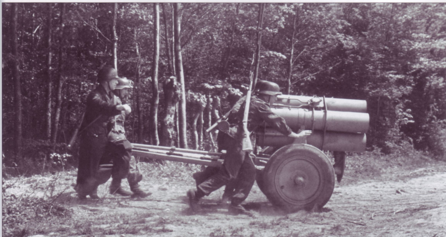
Having only five, instead of the six launch tubes seen on its smaller cousin, this 21cm NbW42 is pushed across a forest track by its crewmembers. The astute observer will note that the wheel and tire arrangement on this carriage matches that of several other German cars, trailers, half-tracks and guns; at least in some cases, there was standardization!
