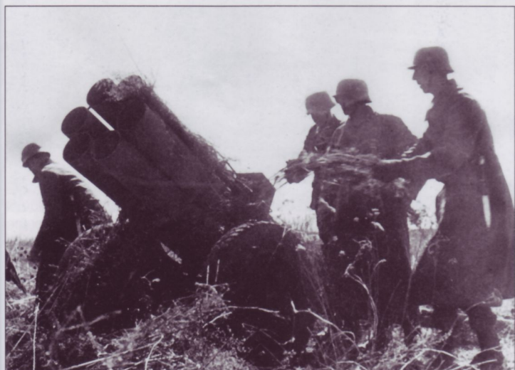
After preparing for a fire mission, this group of soldiers pile local vegetation on top of their 15cm NbW41 to conceal the launcher until the time for its use arrives. The box shape on the launcher covered the electrical junction box to which the remote firing cable was attached.
