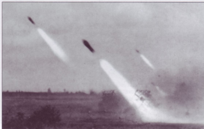
Although Germany used smokeless powder for its guns, rocket propellant was a different matter as this photograph clearly shows. What is possibly a battery of 15cm NbW41s fires a ripple salvo; note the three rockets just leaving the tubes of three different launchers simultaneously, following the smoke trail of the previous three rockets. When all of this ordnance lands down-range, it will devastate the area of the intended target.
