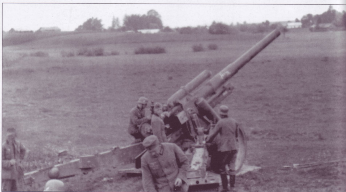
The crew of this 15cm s.FH18 finalizes preparations for a training shoot. Note how a wicker mat has been placed under the carriage's wheels to help prevent them from sinking into the earth, and that the auxiliary hand-crank for the elevation gear has been attached to the trail leg at right.
