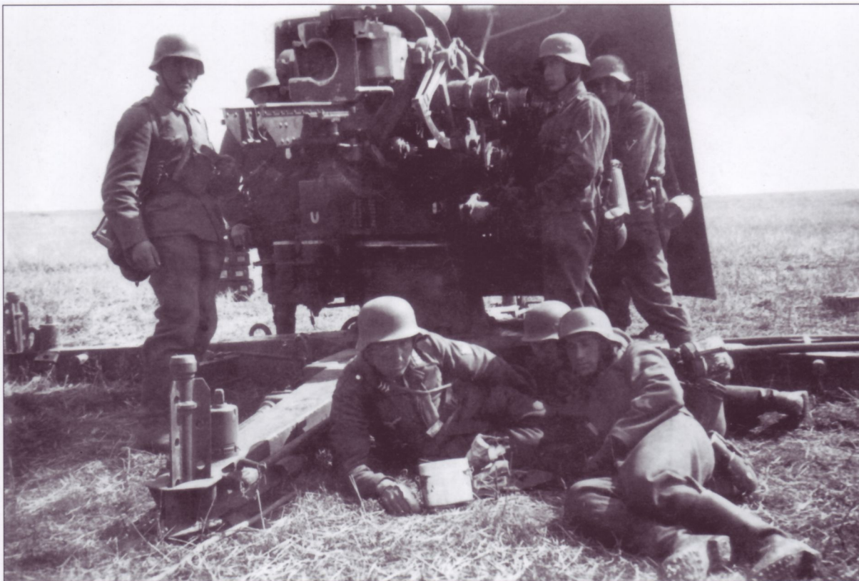
While some of the crewmen stand at their positions, several others have taken a relaxed pose for the photographer of this 8.8cm FlaK36. This Luftwaffe gun is fitted with the Schutzschild (splinter shields); note also the earth anchors used to steady the piece, which are placed at each end of the cruciform gun mount. Their positions denote the Kreuzlafette 36, which identifies this particular model of gun.
