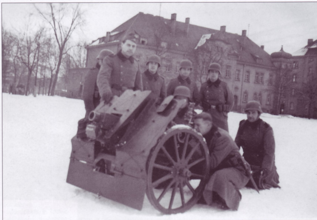
The crew of this 7.5cm I.G.18 poses with their piece against a snowy background. Note the wire running from the bolts that secured the spaced-armor shield in place; this was used to hold foliage in place to better conceal the gun during action. This gun mounts wooden spoke wheels, typical of a piece that was horse-drawn in an Infanterie-Division.
