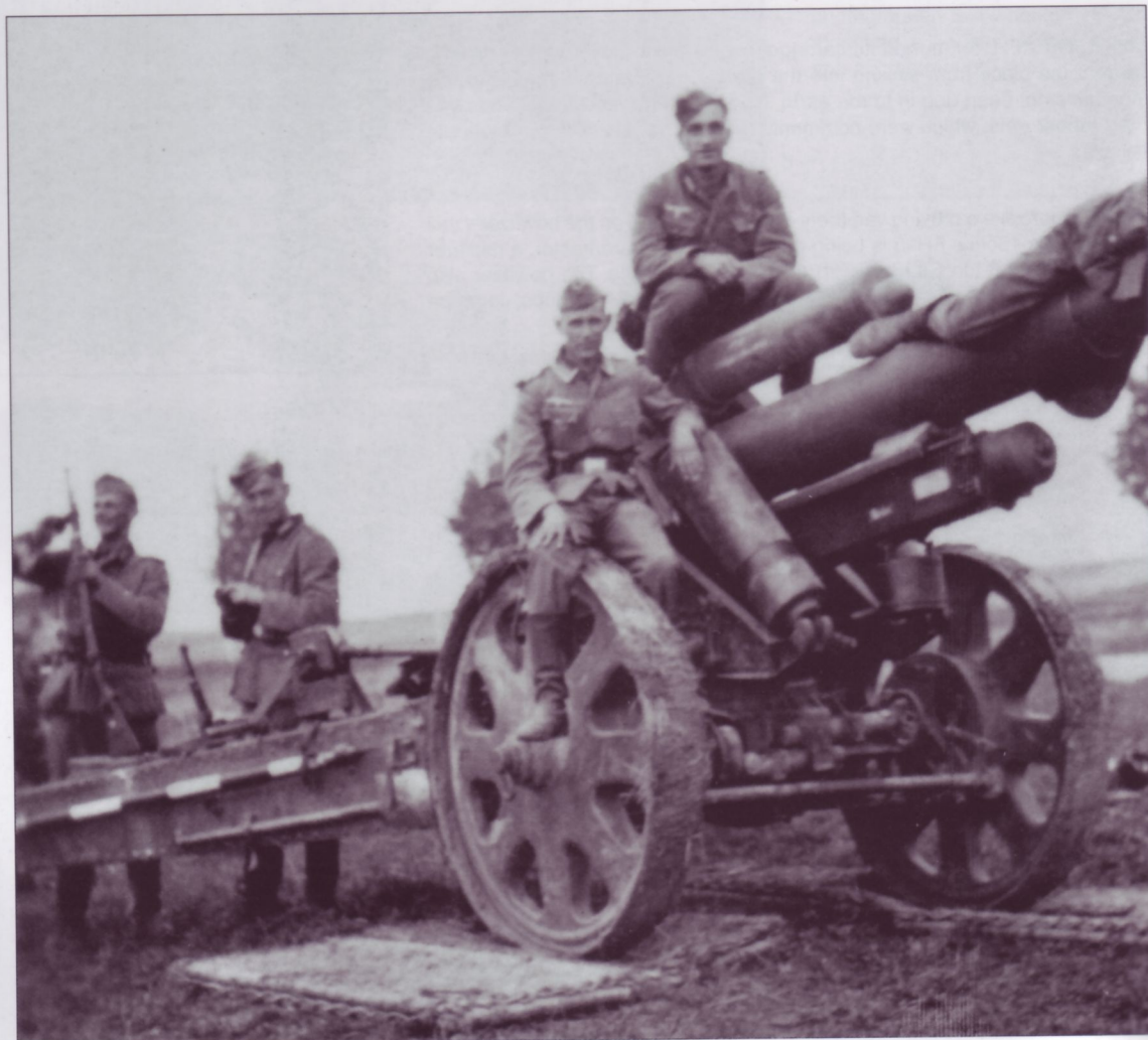
The Heer (Army) crewmen of this 15cm s.FH18 pose somewhat playfully for the photographer. Note the wicker mats placed under the wheels for better flotation on soft ground as well as the shovel and aiming stake stowed on the trail leg; the auxiliary hand-crank for the elevation gear has been mounted above them.
