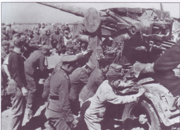
The crew of this 8.8cm FlaK18 struggles to get their piece ready to be emplaced or for travel; note the Sd.Kfz.7 tractor in the background. The FlaK18 was mounted on the Kreuzlafette 18, which was easily recognized by the round leveling pads on the legs, as seen here. This piece also mounts a mono-block gun tube.
