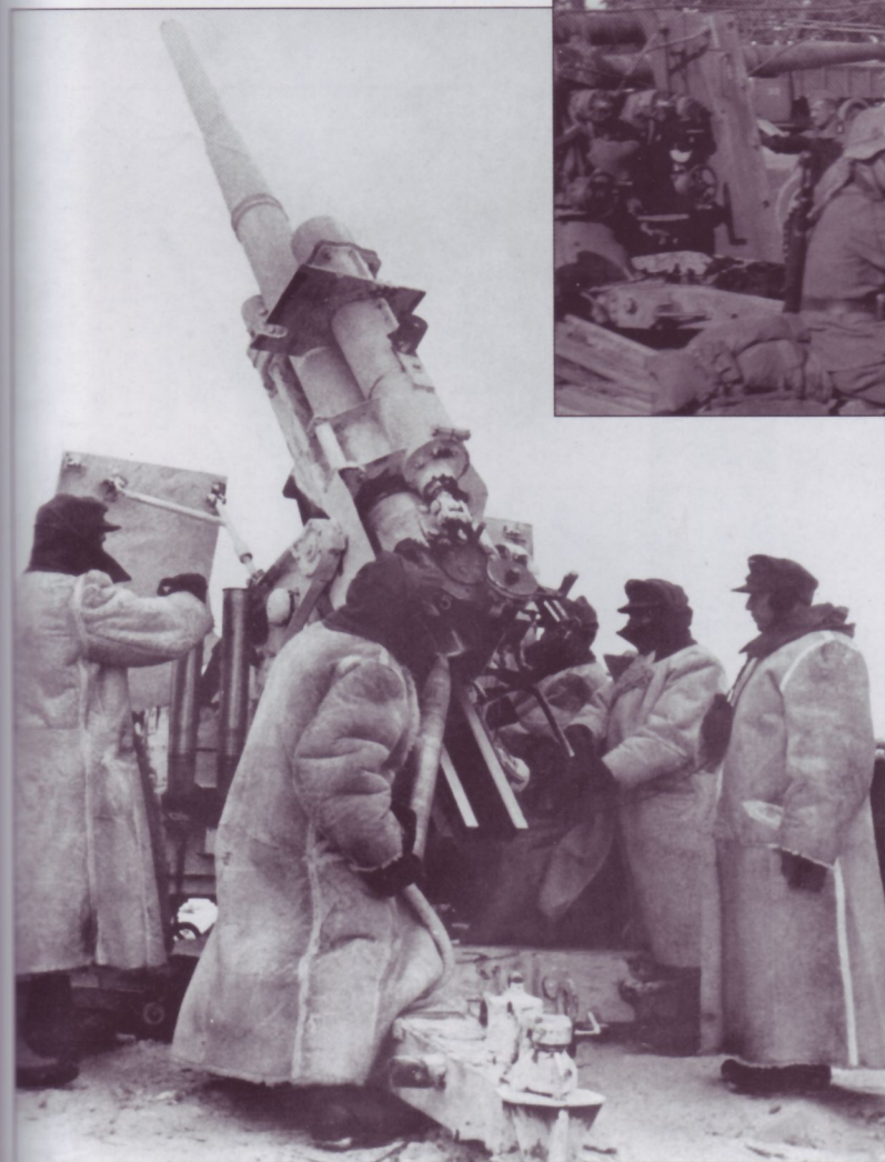
This 8.8cm FlaK18 or 36 guards a road while a column of trucks passes by. Note the round dials of the Lampenempfänger (light signal receiver) which identifies the type. The Schutzschild (splinter shields) lacks the triangular side extensions, but it does mount a framework above it in order to place camouflage materials.
