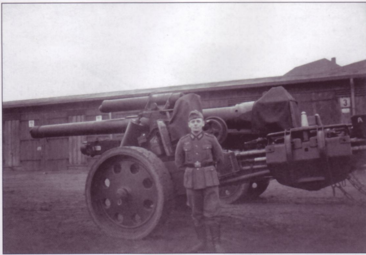
A lone Heer (Army) artilleryman proudly stands before his 15cm s.FH18. A number of interesting features are depicted including the covers over the muzzle, breech and sights; earth spades stored on the trail legs (note the small gun-in-battery letter "A" on the item behind the near spade), and the small data plate on the recoil slide. Compare the perforated wheel style on the carriage to the star-shaped type seen in a previous photograph.
