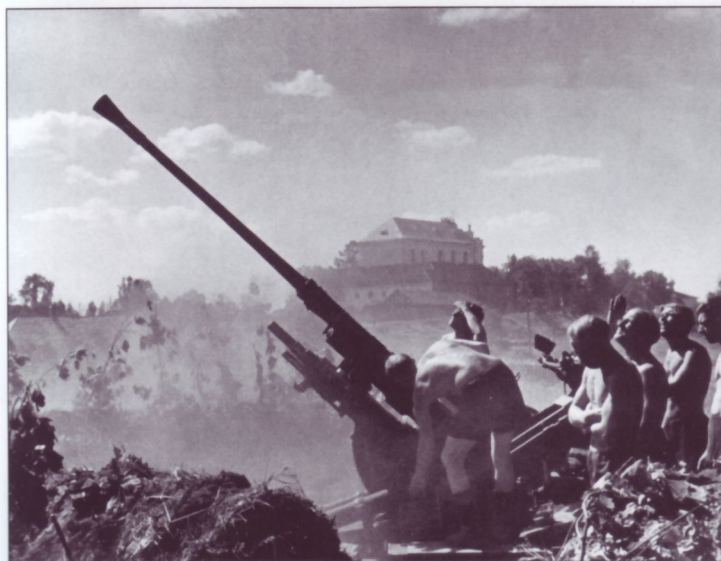
Another group of lightly-dressed crewmen scan the sky while gathered next to their 3.7cm FlaK36. They are located near a built-up area, which may hold a headquarters unit of a logistics center, which is typically where a medium FlaK gun such as this would be deployed. Note that the gun has been dug in and that vegetation has been spread around the parapet to make the turned earth less conspicuous.
