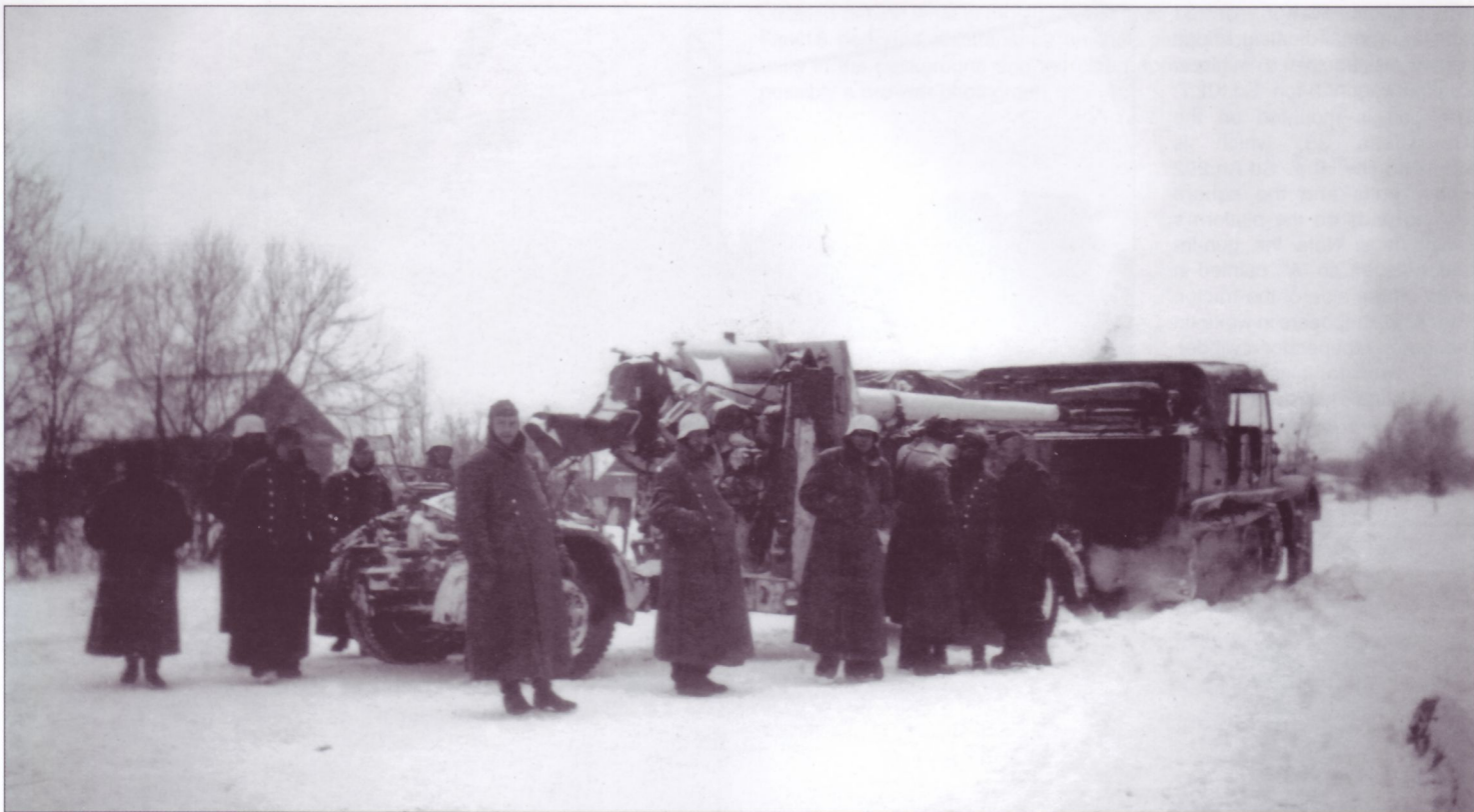
Standing about their 8.8cm FlaK36 and mittlerer Zugkraftwagen 8-ton Sd.Kfz.7, this gun crew stretches their legs in the Russian snow. The gun is identified as a FlaK36 by the circular Lampenempfänger (light signal receiver) dials, as well as the square leveling pads on the legs of the Kreuzlafette 36 cruciform mount. This gun also has Schutzschild (splinter shields) and mounts the mono-block gun tube.
