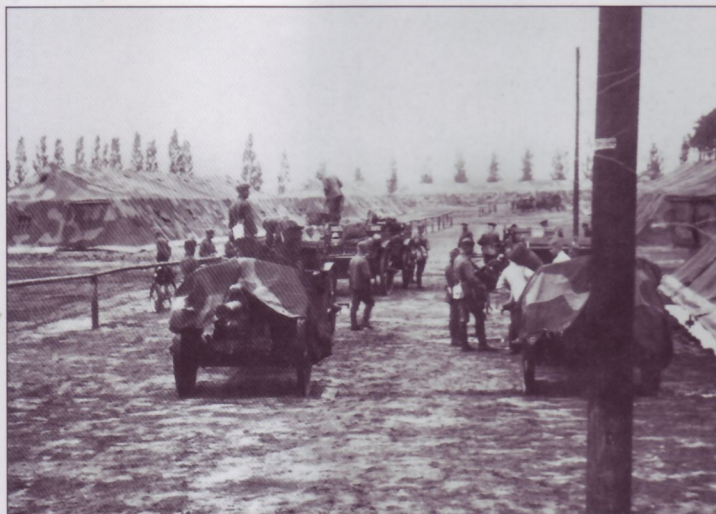
Probably the most interesting parts of this photograph are the distinct camouflage patterns printed on the canvas gun covers and the tents that surround this line-up of horse-drawn 10.5cm I.FH18s. The horses have been un-hitched and the howitzers have been left still attached to their limbers, in this pre-war camp setting.
