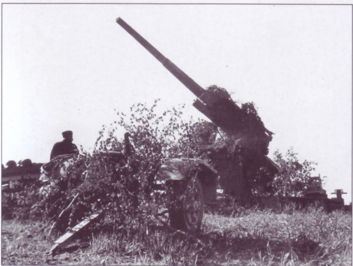
A Luftwaffe officer poses proudly next to his 8.8cm FlaK18, which is being carried on a rail-road flat car. The gun is recognized as a FlaK18 by the round leveling pads of the Kreuzlafette 18. Note the cover over the breech end of this typically clean gun as well as the crewmen's personal equipment and gear laying about.
