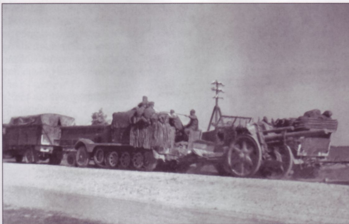
A leichter Zugkraftwagen 3-ton Sd.Kfz.11 moves at speed along a road, hauling a 10.5cm I.FH18 configured for motorized transport. Note the wheel/tire combination and the barely discernable electric brake lamp, on the lower left side of the Schutzschild (splinter shields), just above the folding segment. Note how the latter is folded up for travel, allowing for proper clearance.
