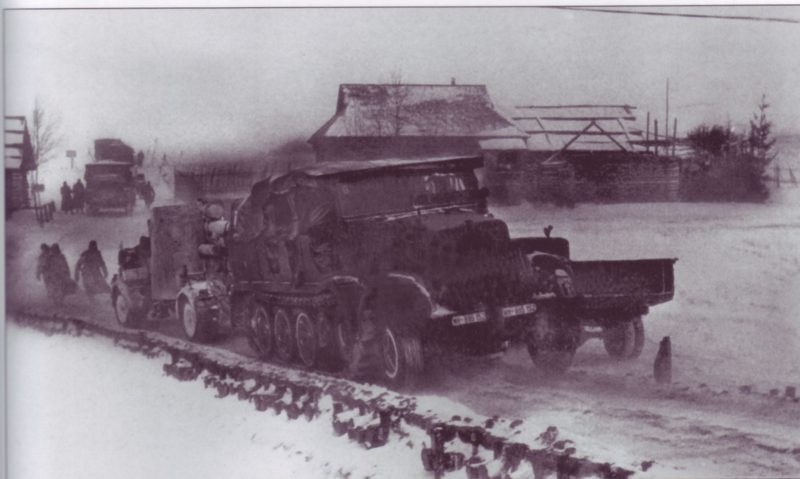
Making its way through absolutely horrid weather conditions, this Heer (Army) 8.8cm FlaK18 is being hauled behind its mittlerer Zugkraftwagen 8-ton Sd.Kfz.7. The tractor exhibits the "Stalhelm" insignia of the Großdeutschland (Greater Germany) Division on its Dunkelgrau RAL 7021 paint finish; below that is the tactical sign for a motorized anti-aircraft unit. The piece is identified as a FlaK18 by the Sd.Ah.201 limber system and the forward orientation of the gun tube while in travel mode.
