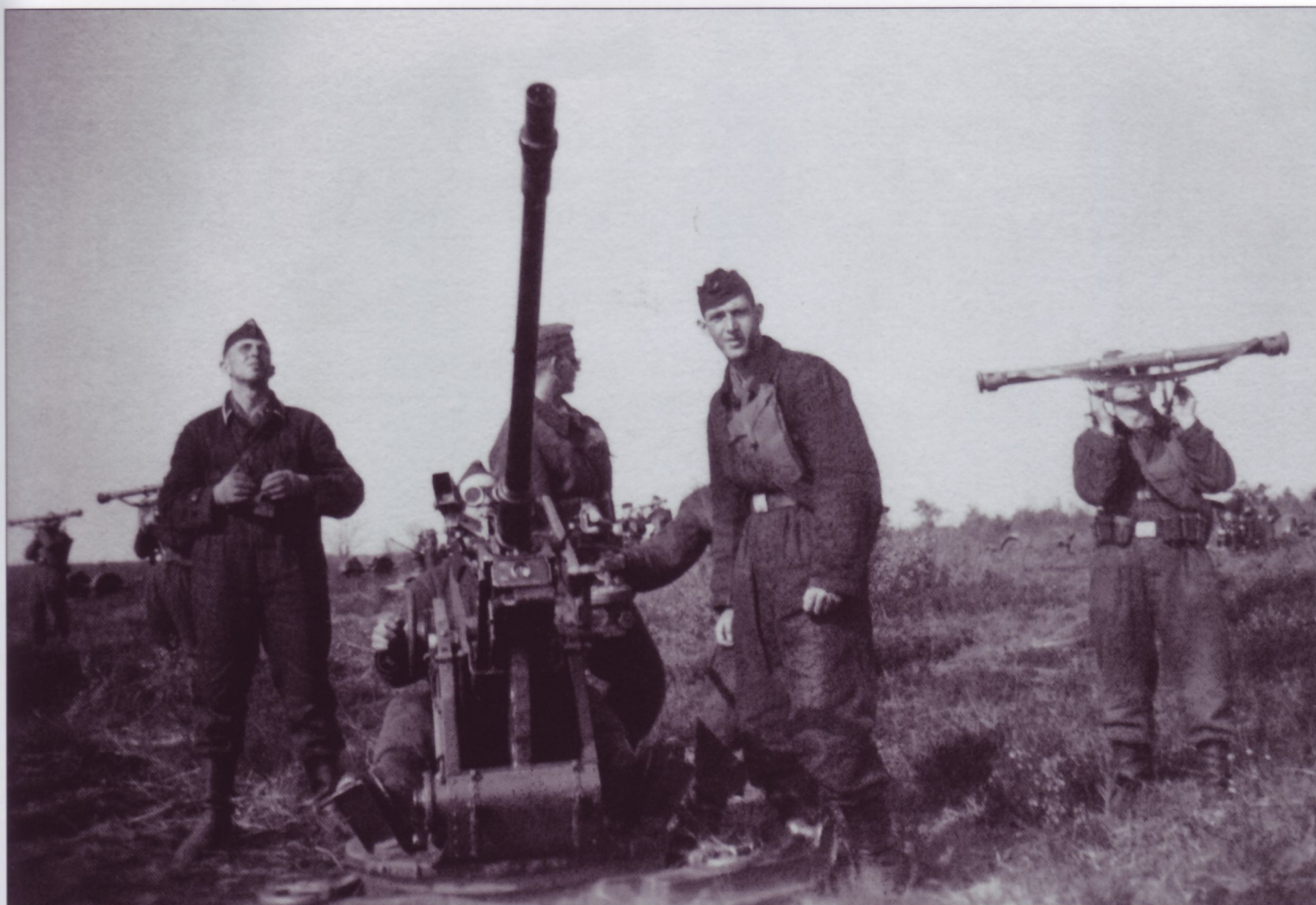
What appears to be an entire battery of 2cm FlaK30s is deployed in an open field. Note the Sd.Ah.51 limbers in the far left background and several men holding 1-meter R36 rangefinders. This Luftwaffe crew wears coveralls and side-caps as well as gas cape pouches slung in front of their chests.
