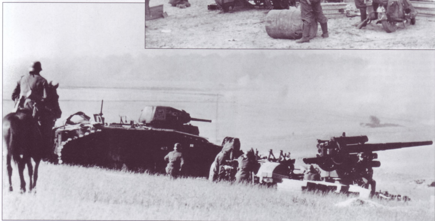
Presumably photographed during the French Campaign of 1940, this 8.8cm FlaK18 uses a destroyed French Char B1 bis heavy tank as cover. The gun is identified as a FlaK18 by the Sd.Ah.201 limber units; it has no Schutzschild (splinter shields) and mounts the mono-block gun tube.
