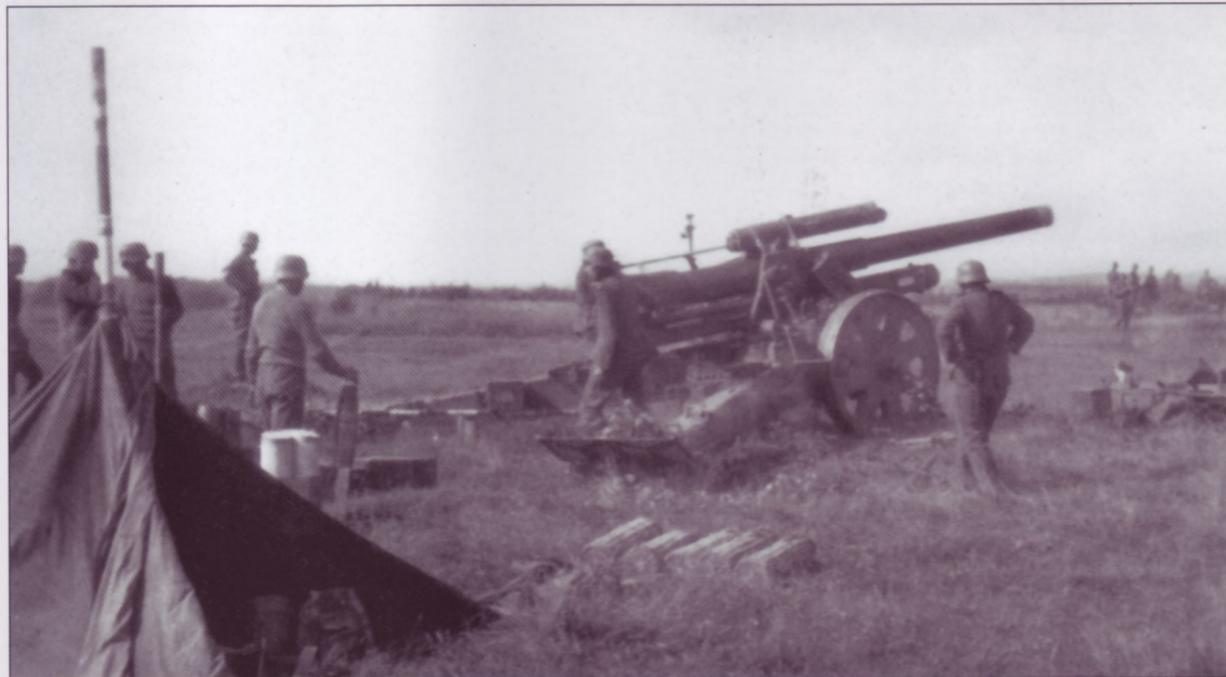
A lone Heer (Army) artilleryman proudly stands before his 15cm s.FH18. A number of interesting features are depicted including the covers over the muzzle, breech and sights; earth spades stored on the trail legs (note the small gun-in-battery letter "A" on the item behind the near spade), and the small data plate on the recoil slide. Compare the perforated wheel style on the carriage to the star-shaped type seen in a previous photograph.
