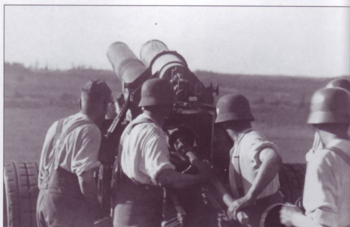
While two men ram the powder charge into the breech of this 15cm s.FH18, another holds the cartridge case for the separate-loading ammunition. With a sliding wedge-type breech block, a case was needed to completely seal that end of the gun tube to prevent the escape of gasses created during firing. A screw-type breech, such as that used on the contemporary US 155mm Howitzer M1, operated in the way its name implied; this provided proper sealing without the need of a cartridge case.
