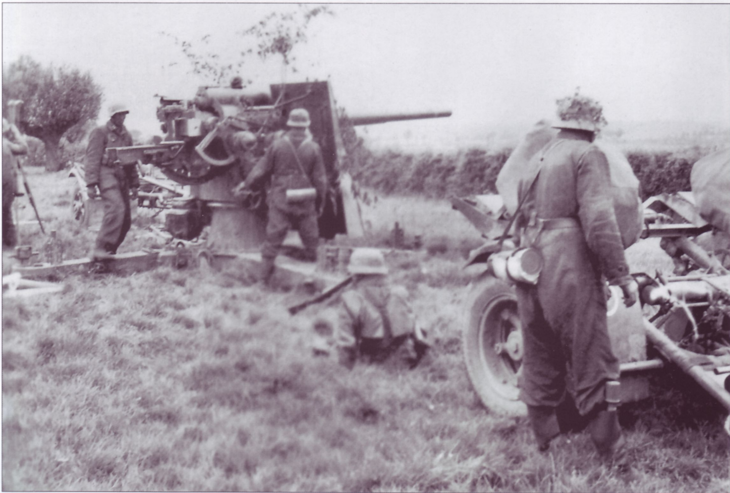
The crew of this 8.8cm FlaK18 engages ground targets with the aid of an observer using a tripod-mounted Scherenfernrohr scissors periscope. The Sd.Ah.201 limber system (one segment in the foreground, the other behind the man in the loader's position) identifies the gun as a FlaK18. Note also the covers over the Lampenempfänger (light signal receiver) dials, which would not be used when the gun was firing at a ground target.
