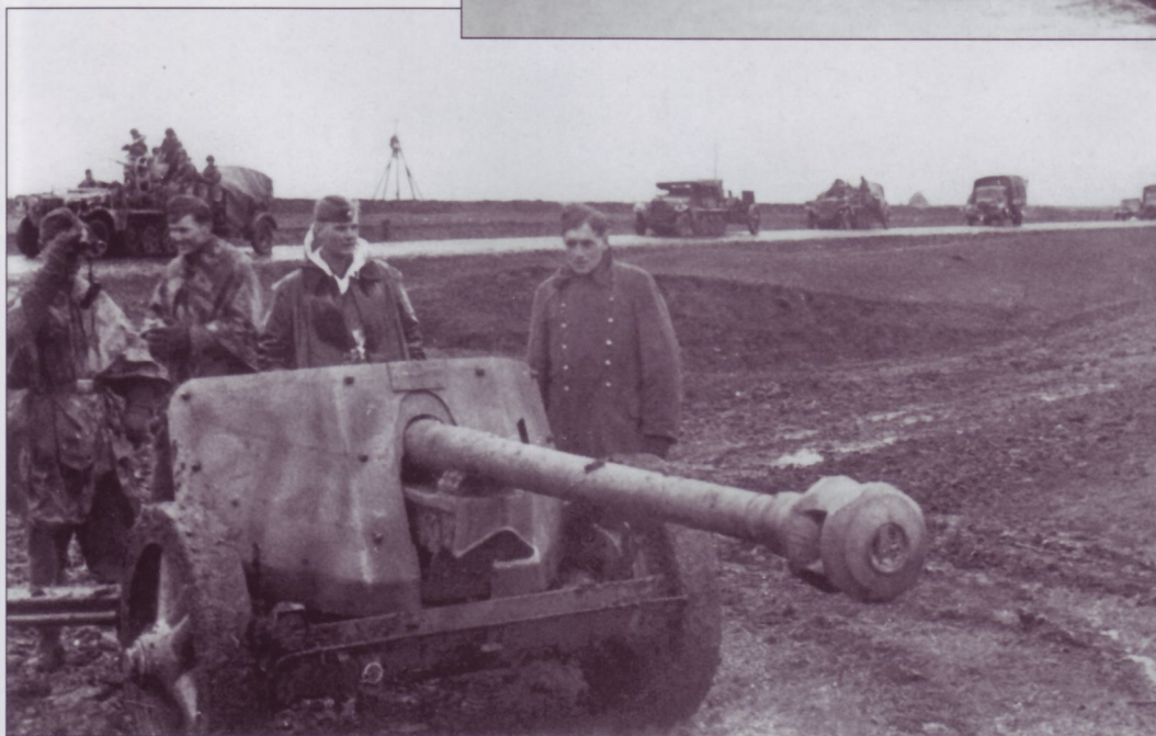
Attached to an un-seen tractor, this 7.5cm PaK40 is configured in travel mode. Note, as was the case with the PaK38 seen in a previous image, how the recoil slide is clamped transversely to the closed trail legs. However, in this case, the gun tube has not been retracted to shorten the piece's overall length for ease in handling tight turns. The wheeled vehicle in the background is a Mercedes-Benz L1500A medium cross-country car.
