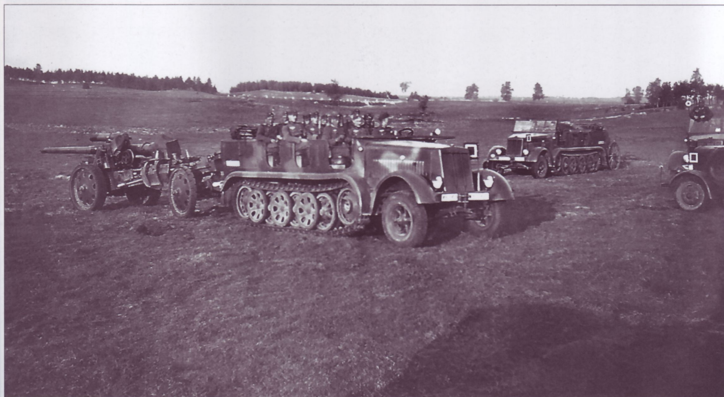
A pristine mittlerer Zugkraftwagen 8-ton Sd.Kfz.7 hauls an equally clean 10cm K18 gun during pre-war exercises. Both the tractor and the gun are painted in the standard pre-war "feuersicherem Buntfarbenanstrich" three-tone system of Nr.17 Erdgelb-matt, Nr.28 Grün-matt and Nr.18 Braun-matt; the tractor's scheme is spray-painted with soft edges, while that on the gun is hand-painted leaving hard edges between the colors. Note that the tractor (it has the KMm11 body style) displays registration plates in the standard positions for the era and that there is also a pennant on the far fender.
