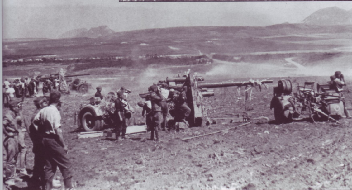
A pair of "eighty-eights", the nearest of which is identified as a FlaK36 by the covered Lampenempfänger (light signal receiver) dials, engages ground targets; the casual appearance of the bystanders suggests that this may be a training shoot. Note that although the guns are positioned on open ground, some attempt has still been made to disguise their outlines with vegetation secured to the gun tubes and splinter shields.
