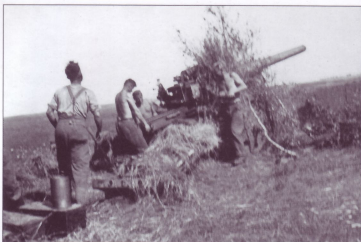
A similar photo of this 15cm s.FH18 appeared in volume one of this series; note how one man is operating the trail leg-mounted auxiliary hand-crank for the elevation gear (at right) and the case for the powder charge laying at far left.
