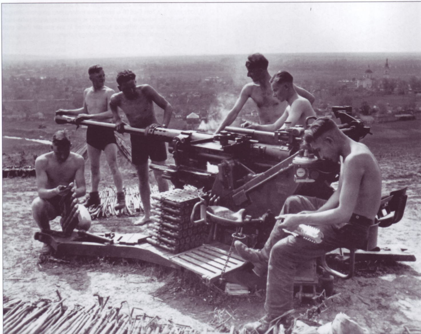
While some men take a break, other crew members of this 3.7cm FlaK36 attend to some maintenance. One man ensures that the clips of ready ammunition are properly cleaned, while the seated man seems to be working with what appears to be the bore swab/brush unit. Note also the small platforms made from thin tree limbs, which would be useful for the crew during wet weather in order to ensure proper footing in action.
