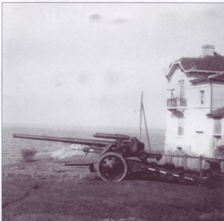
This 10cm K18 has been set up as expedient coast artillery, probably somewhere on the French Atlantic seaboard. Again note the long, thin gun tube, which identifies the type and the very clean appearance of the piece, which is probably painted in the two-tone scheme of Dunkelgrau Nr.46 oversprayed with Dunkelbraun Nr.45 in patches, so the latter color covered roughly 1/3 of the item being painted.
