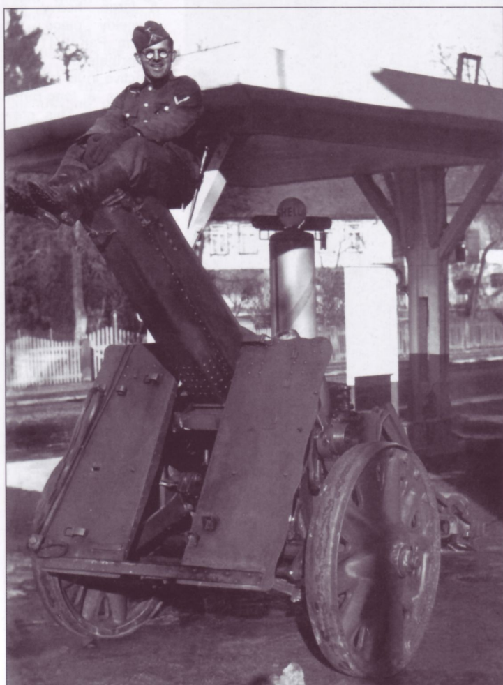
In a pose typical of many artillerymen the world over, this Heer soldier shows off his "big gun" in the form of a 15cm s.I.G.33. This gun is from an Infanterie-Division as can be seen by the cast steel wheels with metal rims; it also lacks the brake lamp seen on the lower part of the shield, which typified guns towed by motorized means.
