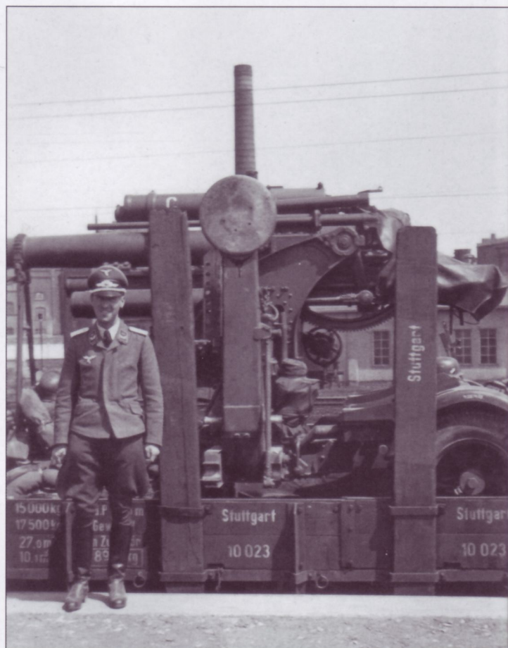
A Luftwaffe officer poses proudly next to his 8.8cm FlaK18, which is being carried on a rail-road flat car. The gun is recognized as a FlaK18 by the round leveling pads of the Kreuzlafette 18. Note the cover over the breech end of this typically clean gun as well as the crewmen's personal equipment and gear laying about.
