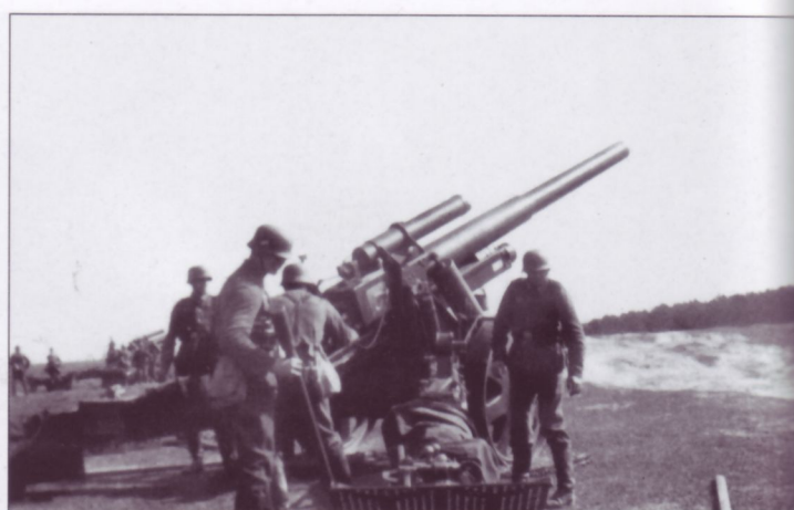
While the gunner prepares to yank the firing lanyard, one of the ammunition handlers stands by with his ramming staff to help feed another round into this 15cm s.FH18. Note that this howitzer, like many others seen in this book, has a data plate on the recoil slide housing and that it also has been fitted with the wheel type associated with a horse-drawn piece.
