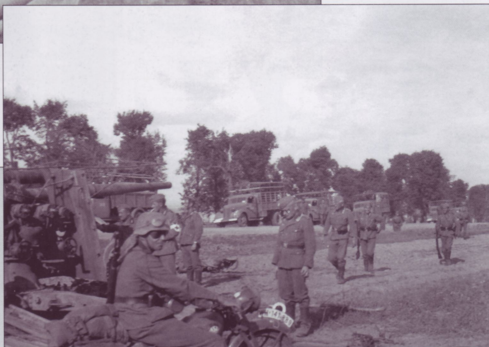
This 8.8cm FlaK18 or 36 guards a road while a column of trucks passes by. Note the round dials of the Lampenempfänger (light signal receiver) which identifies the type. The Schutzschild (splinter shields) lacks the triangular side extensions, but it does mount a framework above it in order to place camouflage materials.
