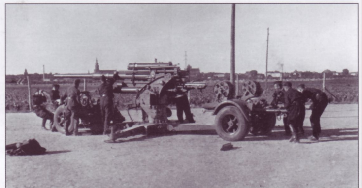
This interesting photograph depicts the crew of an 8.8cm FlaK18 as they either prepare their gun for action, or for transport. Note how the crew manipulates the Sd.Ah.201 limber units, which readily identify this specific sub-type. Note also that it mounts the sectional gun tube, which itself could fit the FlaK18, 36 or 37; the use of this particular item was not an identifying feature of any specific model of the "eighty-eight".
