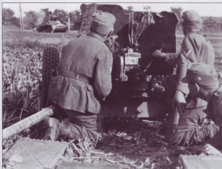
In what is almost certainly a staged propaganda photograph, the Gebirgsjäger crew of this 3.7cm PaK35/36 simulates the close-range destruction of an enemy tank; note the Edelweiss insignia on their trade-mark Bergmütze peaked caps. In this case the "victim" appears to be a Soviet T-26 Model 1939 Light Infantry Tank. With a maximum armor basis of only 25mm, it could be easily penetrated by this gun at ranges in excess of 400-meters.
