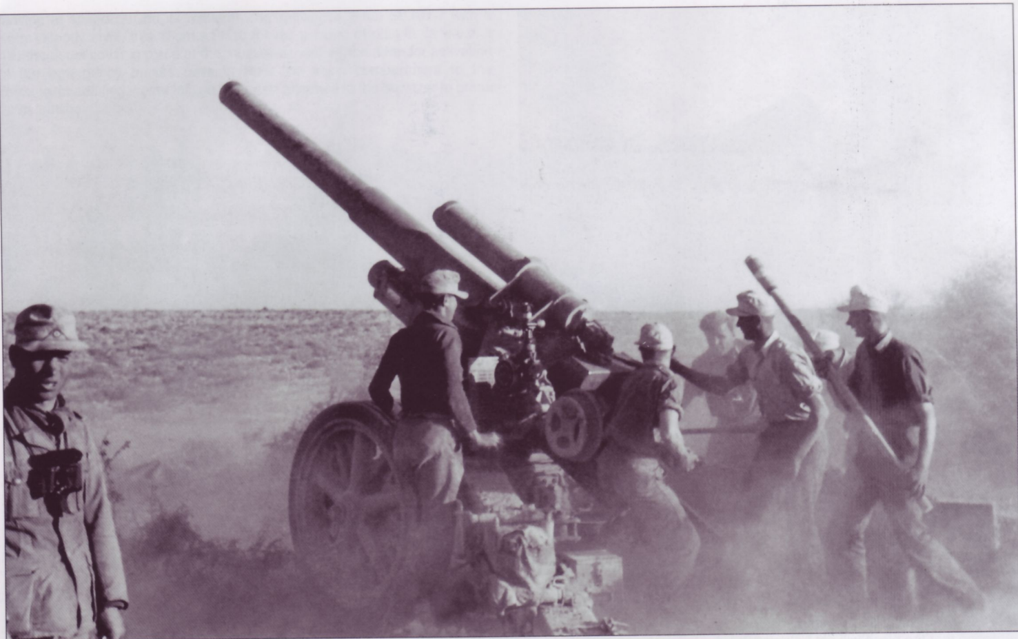
Amid the settling dust created by the firing of the previous round, the crew of this DAK (Deutsches Afrika Korps, German Africa Corps) 15cm s.FH18 prepares to send another shell downrange. Note that this howitzer also has the star-pattern cast wheels with rubber rims, suitable for motorized towing; no horse-drawn pieces served with Rommel's famed desert army.
