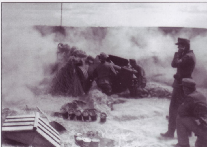
Although they used so-called "smokeless" powder, the shock wave caused by the discharge of this 7.5cm PaK40 has raised a large, tell-tale cloud of dust. One effect of the baffles in the muzzle brake can be noted here in that the dust cloud dissipates to either side of the gun, which the photographer has caught in full recoil. The piece seems to be firing in an indirect role, or at a distant line-of-sight target, judging by the elevation of the gun tube.
