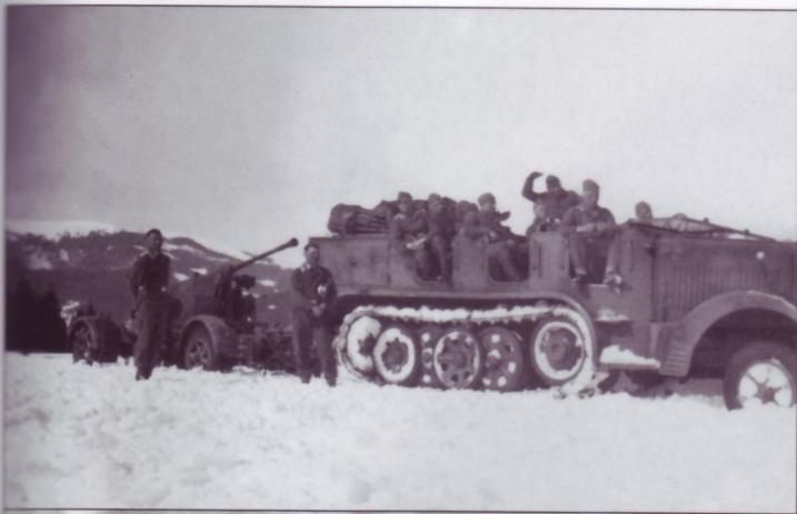
Hauled by an early mittlerer Zugkraftwagen 8-ton Sd.Kfz.7 with the KMm9 or 10 body style, a 3.7cm FlaK18 is seen here moving through snow. The gun is mounted on its twin-axle limber unit and is manned by a Luftwaffe crew. The tractor shows signs of being spray-painted in the pre-war three-color "feuersicherem Buntfarbenanstrich" camouflage scheme.
